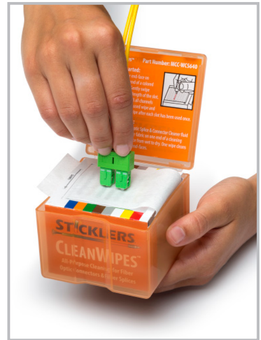
Cleaning slots feature a tight pitch to clean both end-faces on duplex connectors with one swipe.
