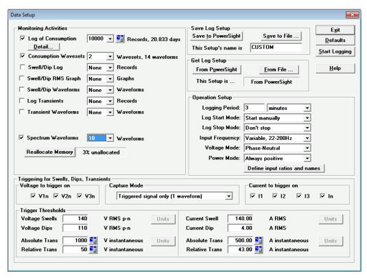
box that says "Spectrum Waveforms", choose how many test you want to allocate to the meter's memory, then press "Save to PowerSight". The amount of tests you can allocate to the meter may vary depending on what memory option you have.
