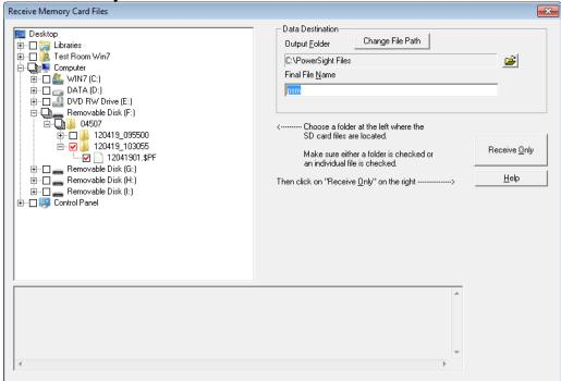
If you took multiple tests with the SD card plugged into your computer, all the tests will be combined into one PFD file, then separated after downloading via the Receive via Memory Card procedure.
