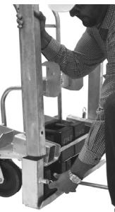
Insert extension legs into operating position by raising plunger pin and sliding leg into socket until plunger pin is fully engaged. Repeat for second leg.
