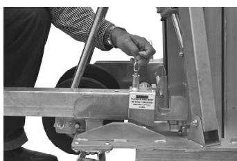
Unlock caster swivel lock on cart to allow rear caster to swivel freely during operation.
