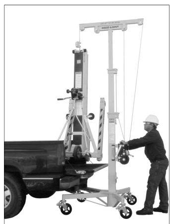
To release Hold Down, pull bar toward you and place back behind mast sections.
