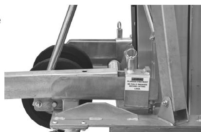
This condition can be corrected using the adjustment knob. First, loosen the lock nut located in the saddle. Turn the large adjustment knob counter clockwise to raise the saddle and clockwise to lower the saddle. Once the saddle is level with the Extension Leg re-tighten the lock nut.
