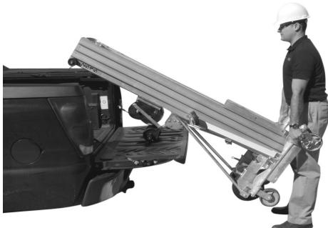
wheels and 10" transport wheels. Tie the unit down to prevent movement during transport. Unit may be loaded with a crane. Unit must be in upright and compact position with legs, forks, and stabilizers securely in their stored positions. If unit has any loose or unsecured items, remove them. Attach to lifting eye located on top of bottom mast. Before elevating unit, lifting hook should always point away from the lift.
