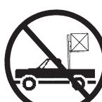
When a unit has an elevated load, it can be transported on the unit's 6" casters only. Do not operate from an unstable platform such as the bed of a truck.
