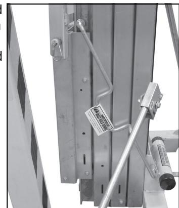
When properly installed, the winch handle should be mounted as shown in the picture with the steering handle in the lowered position. Do not attempt to raise or lower a load with the handle mounted in any other manner.
