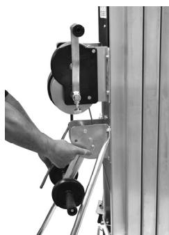
Reverse this procedure to store handle. The handle must be in the stored position to operate the winch.
