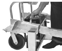
Slide leg lock block to the fully forward position.
