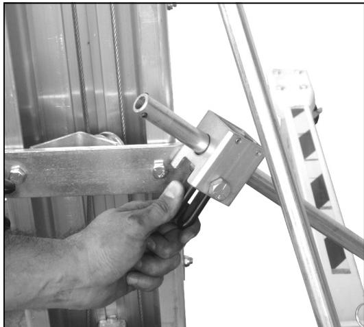
To replace the leg in the stowed position, pinch the locking mechanism release and fold the leg up.
