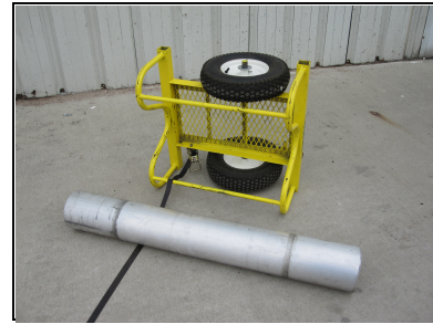
Place strap under pipe by rolling pipe.
