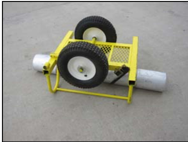
Put Cricket on top of pipe and ratchet strap tightly
