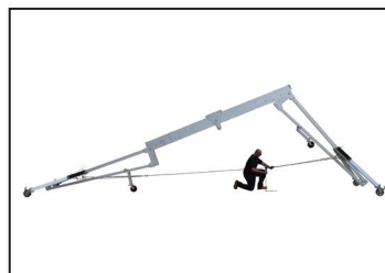
Ratchet 1st A-Frame bolt to beam.
