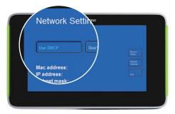
DHCP must provide an IP address, gateway, and domain name or the RoomWizard will reject the DHCP settings. If the RoomWizard rejects the DHCP settings, it will adopt a default static address. You can use this default or another static address to access the RoomWizard's web-based setup pages and enter DHCP settings manually.
