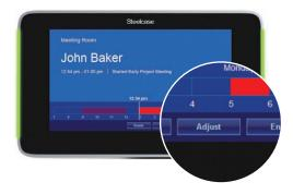
RoomWizard displays the current reservation end time and buttons labeled "+" and "-." Press "+" or "-" to add or remove time from the current reservation.
