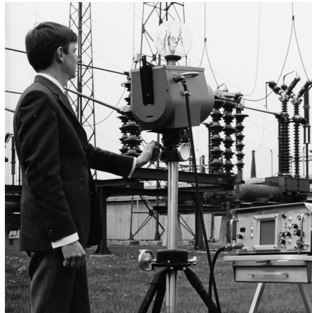
Figure 29.2 1969: Thermovision Model 661. The camera weighed approximately 25 kg (55 lb.), the oscilloscope 20 kg (44 lb.), and the tripod 15 kg (33 lb.). The operator also needed a 220 VAC generator set, and a 10 L (2.6 US gallon) jar with liquid nitrogen. To the left of the oscilloscope the Polaroid attachment (6 kg/13 lb.) can be seen.
