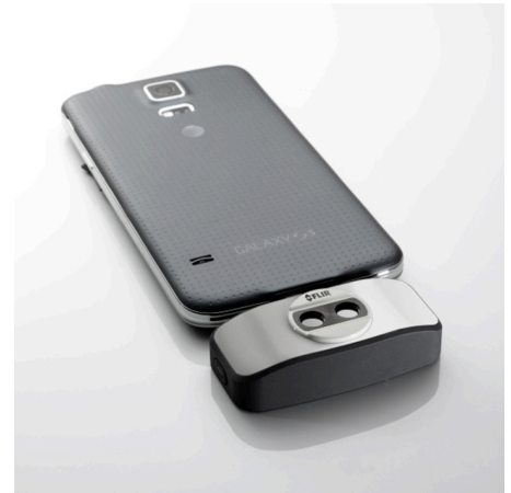
Figure 29.3 2015: FLIR One, an accessory to iPhone and Android mobile phones. Weight: 90 g (3.2 oz.).
