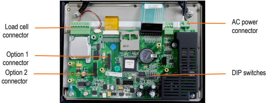
Figure 1-3: T72XW Main Board Connections, AC Model
