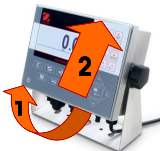
Figure 1-2: Removing the Cover
