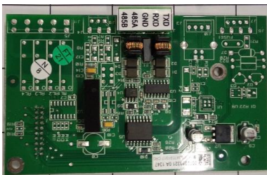
Figure 1-7: COM2 Option Board
