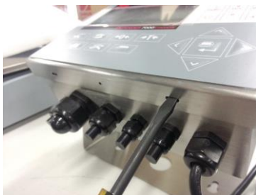
Figure 1-1: Opening the Harsh Enclosure
