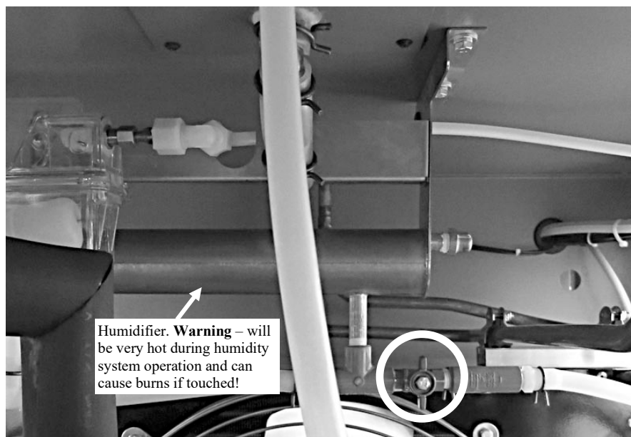
Figure 7-2 – Humidifier Drain Valve (circled, shown in the closed, or normal operating position)
