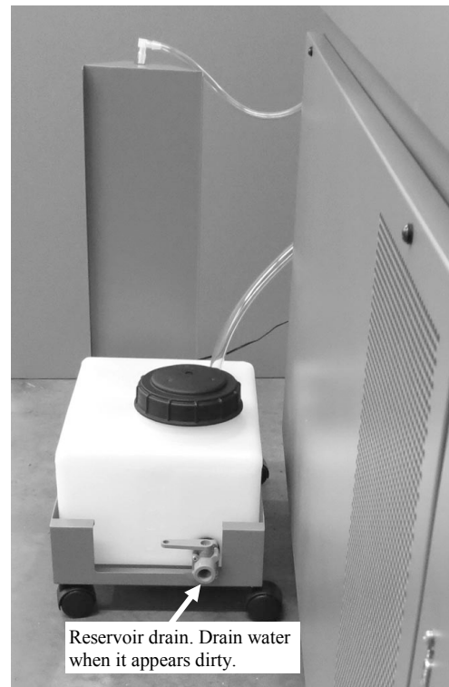
Figure 7-1 – Reservoir Drain Valve
