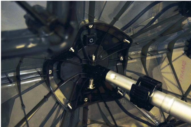
When using the short pole or with the SAH22A adapter base kit for canvas hoods, the stationary pole adapter should be used to keep the pole from pivoting. Place the stationary pole adapter onto the SAH22A and attach using the screws and wing nuts provided (below). Once secure, insert the short pole and secure in place using the locking pin.
