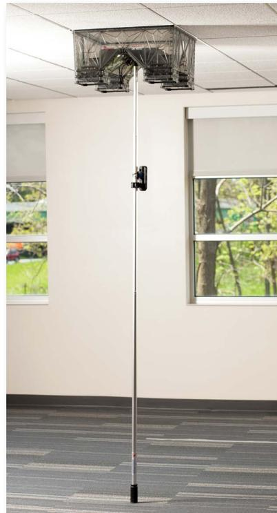
Once the hood is placed correctly, twist the pole to adjust the pole length so that it reaches the floor supporting the hood itself. If the hood is not securely in place, then re-adjust the pole length.
