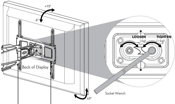
Position your display to the desired viewing angle using the angular movement allowed by the double ball mount.
