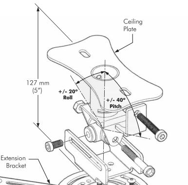
NOTE: 4 sets of Extension Bracket lengths are included to suit most mounting configurations. Any combination of these brackets may be used.
