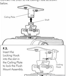
F.3. Tighten the Locking Hook with the M8x50mm Socket Cap Screw and the M8 Nyloc Nut that was previously removed.
