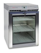
combination of cold-wall and forcedair mechanisms helps ensure that conditions are optimal for the most demanding applications such as vaccine or pharmaceutical storage.
