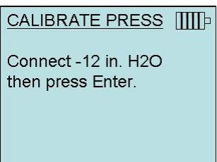
Apply -12 in. H<sub>2</sub>O to the "+" port on the meter under test **OR** apply +12 in. H<sub>2</sub>O to the "-" port
