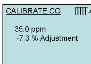
In this example, the span gas is rated at 35 ppm. Use the UP or DOWN arrow keys to adjust offset to match the span gas concentration. Press **ENTER** to accept and to return to the CALIBRATION menu.
