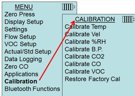
**Notes:** The measurement capabilities of the instrument and probe will determine what appears in the main MENU and CALIBRATION menu. Instrument models using detachable probes must have the probe attached to perform field calibrations. The screen displays used in this document are from the 9565 series VelociCalc® Multi-Function Ventilation Meter.
