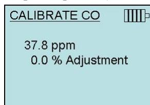
Once the countdown is complete, the CO concentration as measured by the probe is displayed along with the percent of adjustment.
