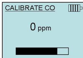
After pressing **ENTER** with the zero calibration gas connected, the instrument will begin to take data. A bar graph will appear showing the time remaining.
