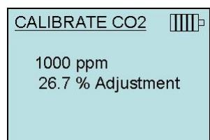
In this example, the span gas is rated at 1000 ppm. Use the UP or DOWN arrow keys to adjust offset to match the span gas concentration. Press **ENTER** to accept and to return to the CALIBRATION menu.
