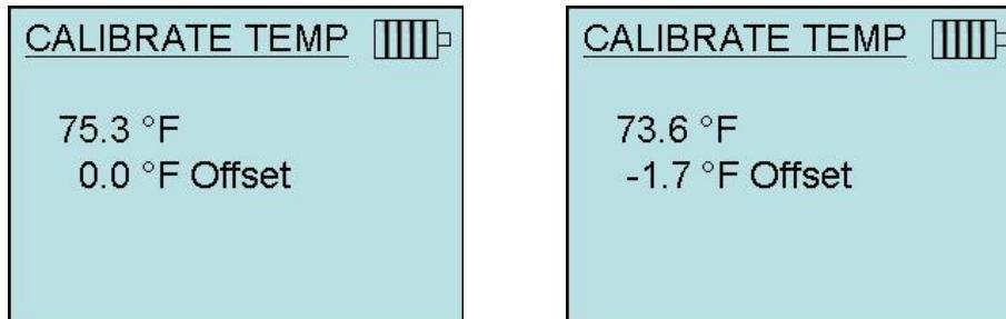
In this example, the temperature measured by the probe is 75.3°F and the reference temperature is 73.6°F. Adjusting the offset by -1.7°F allows the probe match the reference standard.
