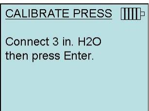
Apply +3 in. H<sub>2</sub>O to the "+" port on the meter under test
