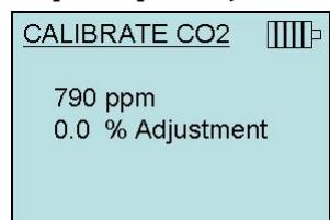
Once the countdown is complete, the CO<sub>2</sub> concentration as measured by the probe is displayed along with the percent of adjustment.
