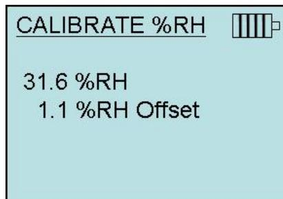
In this example, the relative humidity measured by the probe is 30.5 %RH and the reference humidity is 31.6 %RH. Adjusting the offset by 1.1% allows the probe match the reference standard.
