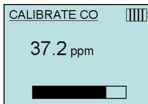
After pressing **ENTER** with the span calibration gas connected, the instrument will begin to take data. A bar graph will appear showing the time remaining.
