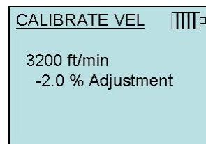
Instrument adjustment using up and down keys. Press **ENTER** to accept.
