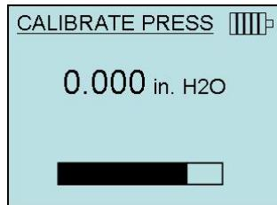
After pressing **ENTER**, the instrument will begin to take data. A bar graph appears showing the time remaining for the zero calibration.
