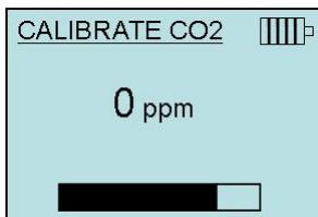
After pressing **ENTER** with the zero calibration gas connected, the instrument will begin to take data. A bar graph will appear showing the time remaining.
