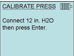
Apply +12 in. H<sub>2</sub>O to the "+" port on the meter under test
