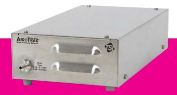
The TSI AeroTrak® High Pressure Diffuser (HPD) Model 7950 and Model 7955 accessories allow the TSI AeroTrak Particle Counters to measure particulate contamination in high-pressure compressed gas systems. As particle counters cannot sample high pressure gas, they require HPD accessories to reduce the pressure of compressed gases to assess the cleanliness level of compressed gas systems.
