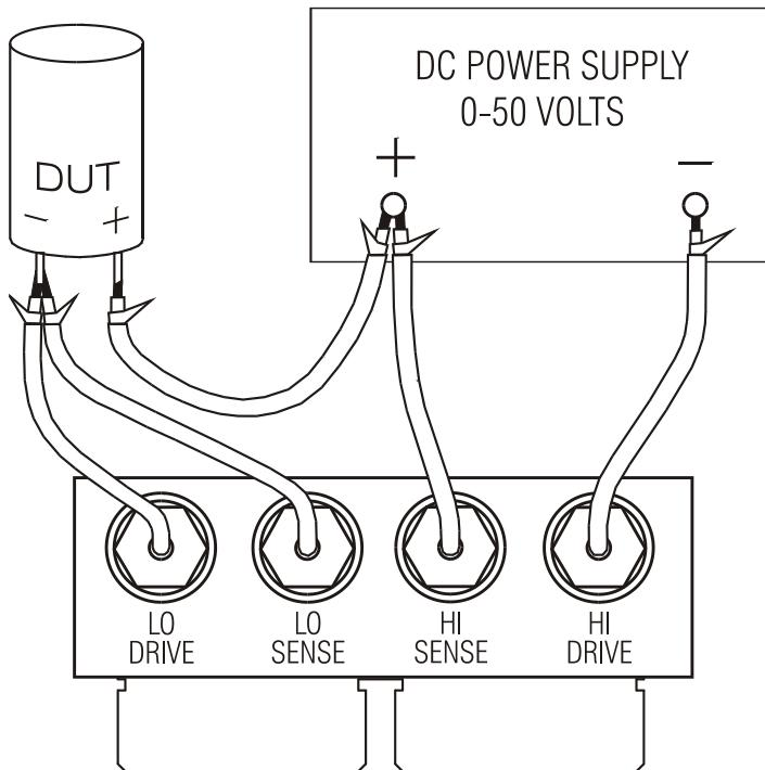
The external DC bias must be connected to the LCR400 and DUT as shown in the diagram. The High Drive, High Sense, Low Drive and Low Sense connections to the LCR400 are made using the optional interface module which inserts into the Kelvin connectors on the top of the instrument.
