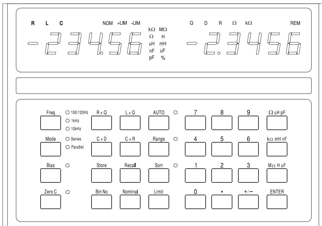
In normal use the left-hand 5-digit display shows the value of the major parameter (L, C or R) and the right-hand display shows the value of the minor parameter (Q, D or R). The parameters being displayed are indicated above their respective numeric values and the units of the parameter are shown to the right of the value itself. A display test which lights all the indicators can be carried out by holding down any key while the instrument is switched on.
