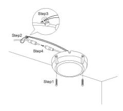
Installation 3 ----- Attach to concrete surface
