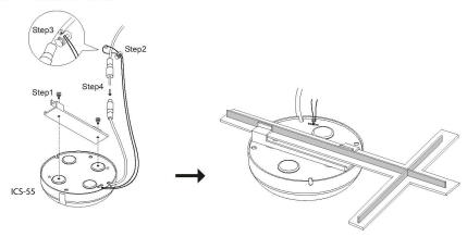
Installation 2 ----- Attach to wood surface
