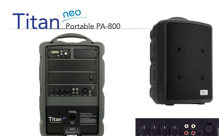
Titan AC/Battery powered portable sound system (basic unit). The Input Panel provides a Lo-z XLR Microphone Input with Volume Control, Stereo Line Input with volume control and Dual Line Output, Treble & Bass Controls, Master Volume Control. Voice Priority Circuit and Battery Level Indicator.
