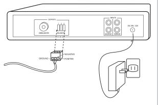
Plug power supply into AC outlet. Plug power cable into receiver.
