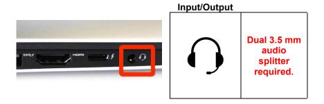
3. <u>USB connection</u>: If the computer does not have 3.5 mm connections, connect to the computer's USB port using a USB-to-3.5 mm splitter.
