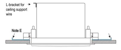
STEP 7. Take care to connect the wire on + terminal of amplifier to + terminal on speaker and the other wire likewise to - terminals. For best connection, use spade terminals (18 gauge) on wire ends connected to speaker. Once connected, replace ceiling tile into ceiling.
