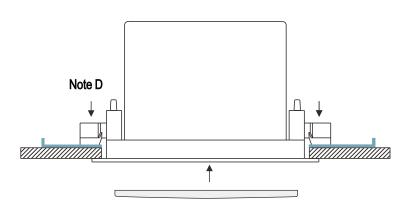
STEP 8. Where required by code or construction standards, connect support wire from structure above ceiling to speaker L-bracket and tile bridge through provided support locations as show in **Note E**.
