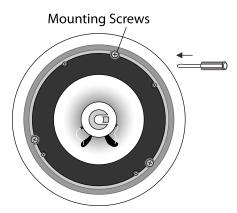
STEP6. As the screws are tightened, the tabs will turn outward then begin descending to engage and press against the mounting surface as in **Note D**. Take care to see that they turn out and do not bind before sandwiching the tile bridge and the ceiling tile between the tabs and the speaker front flange. Do not over tighten. After all three screws are tightened and the mounting is secure, reinstall the speaker mesh grill.
