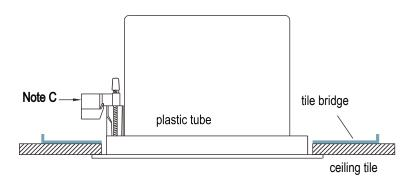
STEP 5. Secure the speaker to the ceiling tile by tightening the three tabs. THE POSITION OF THE THREE TABS SHOULD BE LOCATED ON TOP OF THE THREE TUBES as shown at **Note C** on the drawing prior to tightening. Tighten the three screws one by one.
