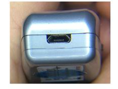
The shape of the plug is not symmetrical, and the cord's plug can go in only one way.
