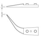
Tip dimensions: A (tip thickness) B (tip width)
