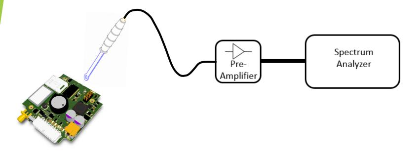
Localize the source of unwanted emissions on the DUT PCB using near field probes and a spectrum analyzer.
