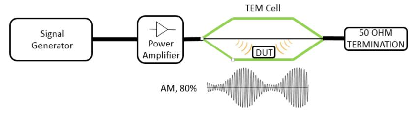
Terminate any of the two ports of the TEM cell with the  $50\Omega$  load, and connect the signal generator + power amplifier to the other port. The signal needs to be AM modulated (80%) according to most standards. The power of the signal has to be chosen according to the required field strength. Place the DUT under the septum and power it on.
