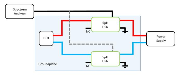
The DUT shall be isolated and elevated from the groundplane. The spectrum analyzer shall measure the conducted emissions on both supply lines. The RF output of the unused LISN shall be terminated with 50 Ohm. If the power return line is less than 2 m, a setup with a single LISN is sufficient. For the exact details of the set up and for the limits of conducted emissions refer to the CISPR 25 or relevant applicable standard.
