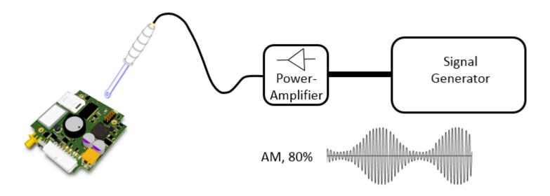
Localize the section on the DUT PCB which is susceptible to RF.
