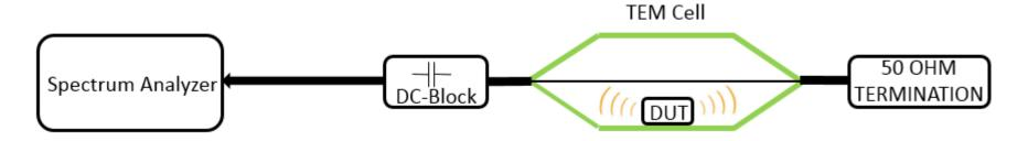
Terminate any of the two ports of the TEM cell with the  $50\Omega$  load, connect the DC-Block to the other port and connect it to the input of the spectrum analyzer. Place the DUT under the septum and power it on.
