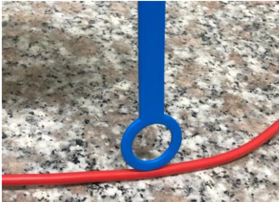
Picture 1: Correct positioning of the H-field probe
