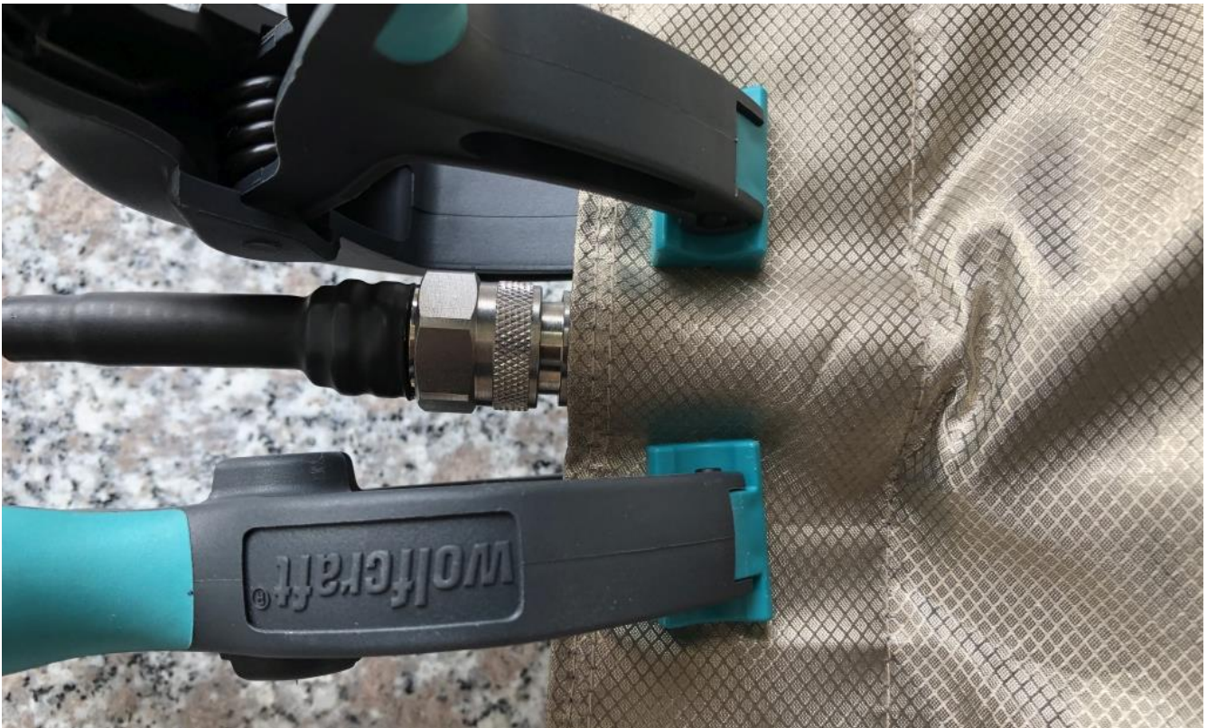
Picture 13: feed through at the DC-block of a TEM-cell; bag closed
