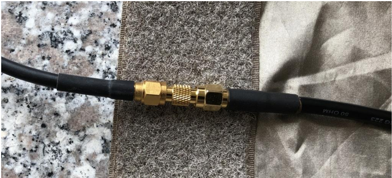
Picture 9: feed through using coaxial adapter
