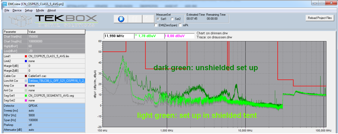
Picture 6: CISPR 25 conducted noise measurement; DUT powered
