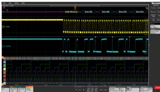
I 2 C decoding synchronized with digital waveforms from a TLA058 logic probe
