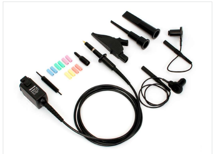
Figure 5. Tektronix TPP0850 Voltage Probe. Single-ended, ground-referenced probe with 50x attenuation (up to 100V RMS ) and 800 MHz bandwidth.
