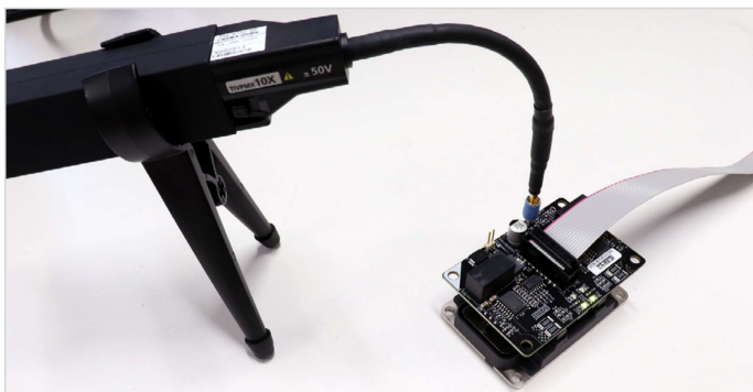
Figure 15. Square pin style sensor tip cables. Photo © Wolfspeed. Reprinted with permission.
