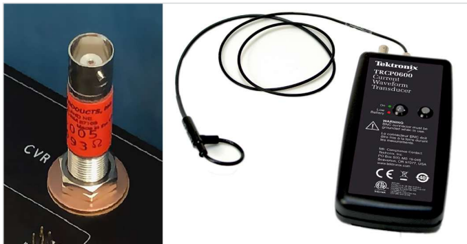
Figure 7. Probe examples, (a) Current Viewing Resistor (T & M Research SSDN-005, 400 MHz). Photo © Wolfspeed. Reprinted with permission. (b) Rogowski Current Probe (TRCP0600 Current Waveform Transducer, 30 MHz).
