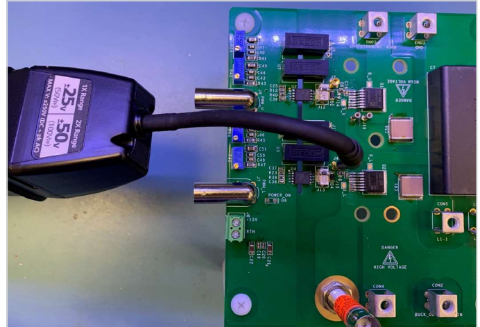
Figure 13. MMCX connectors - Example 2. Photo © Wolfspeed. Reprinted with permission.
