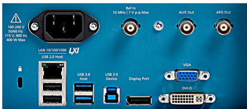
Figure 32: The I/O you need to connect the 5 Series MSO to the rest of your design environment.
