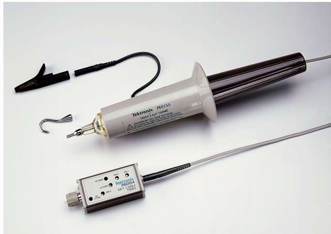
Figure 2.5. High-voltage probes can measure DC voltages up to 20 kV and pulses up to 40 kV with a bandwidth of 75 MHz.
