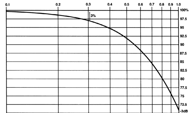
Figure 4.8. Bandwidth derating curve.
