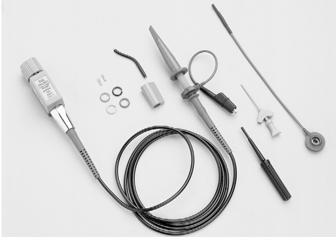
Figure 2.14. A typical general-purpose voltage probe with its standard accessories.
