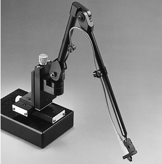
Figure 2.10. Example of a probing station designed for probing small geometry devices such as hybrid circuits and ICs.
