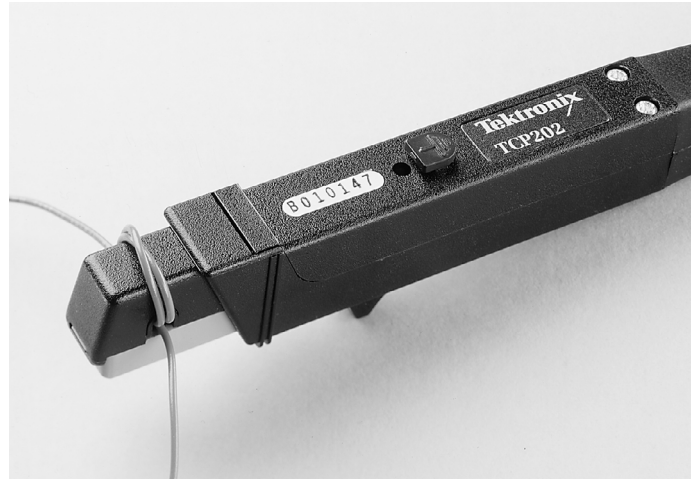
Figure 2.8. An example of a split core AC current probe. Looping n turns of the conductor through the probe increases effective sensitivity n times.
