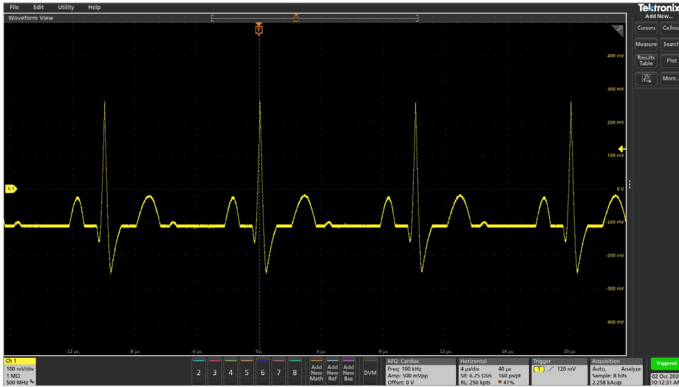
Figure 12: Simulated heartbeat waveform captured on the Tektronix MSO5 Oscilloscope.
