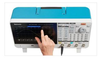
The large capacitive touchscreen and built-in ArbBuilder tool enable users to create and edit arbitrary waveforms right on the instrument.
