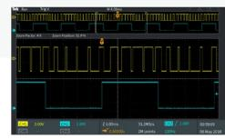
Since an oscilloscope can store only a limited number of samples, the waveform duration (time) will be inversely proportional to the oscilloscope's sample rate. Time Interval = Record Length / Sample Rate
