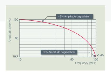
Bandwidth is defined as the frequency at which a sine-wave input signal is attenuated to 70.7% of its true amplitude (the -3 dB or 'half-power' point, shown here for a 100 MHz scope).
