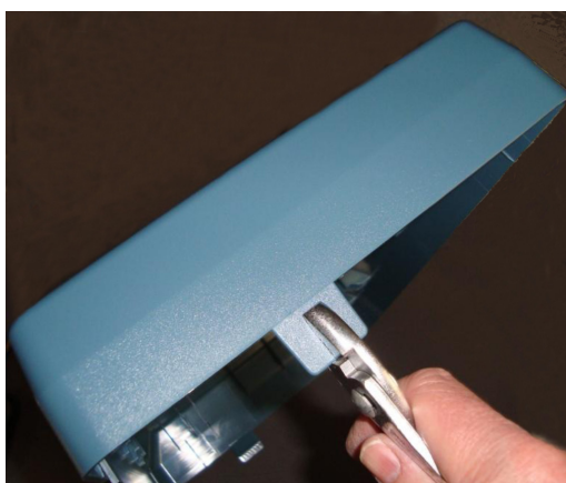
Figure 2: Removing tabs from the front protective cover
