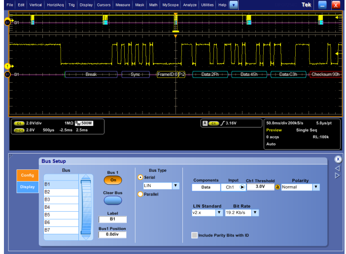
LIN bus setup, showing assignment of source, thresholds, standard, and bit rate.
