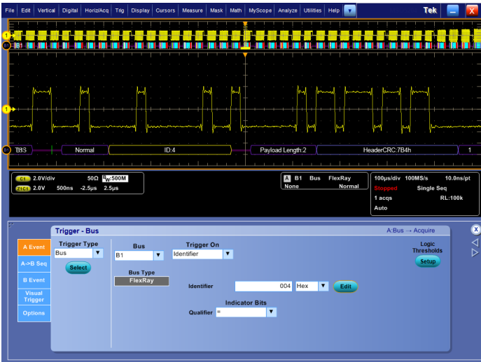
Triggering on a specific Identifier value on the FlexRay bus.
