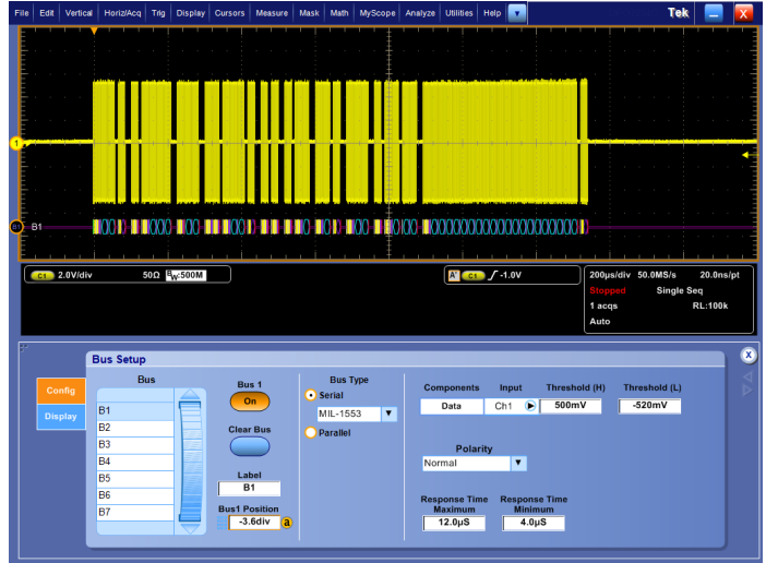
MIL-1553 bus setup, showing dual threshold settings.
