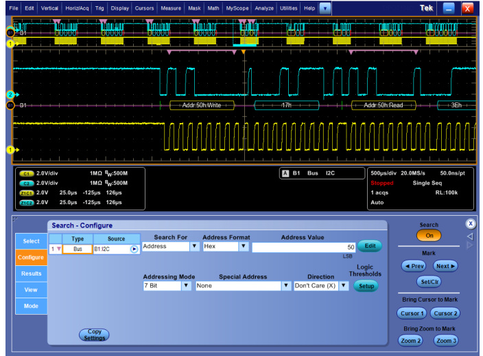
Serial Search display showing every occurrence of the specified serial event.
