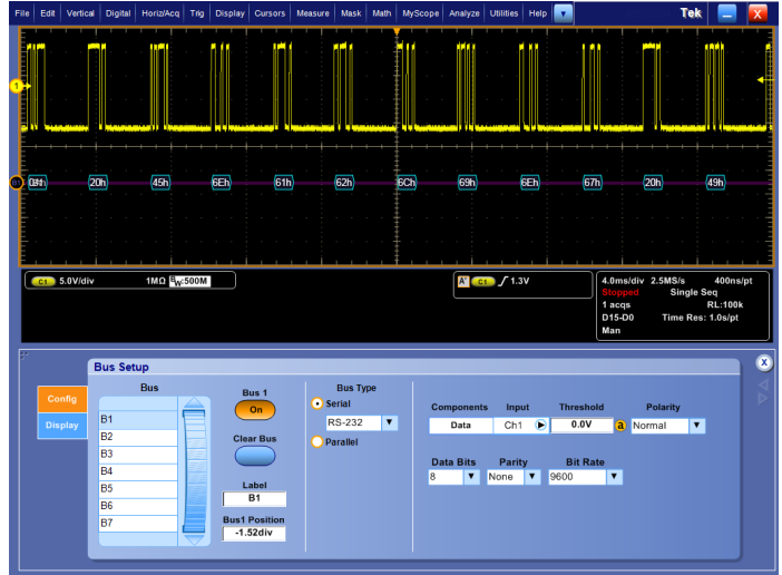
RS-232 bus setup, showing assignment of source signal, digital threshold, and polarity.
