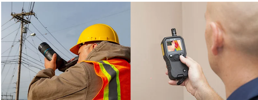
FOV determines how much the camera sees and from what distance. A telephoto lens is better for measuring at a distance (left), while a wide angle lens is better for close-up work (right).
