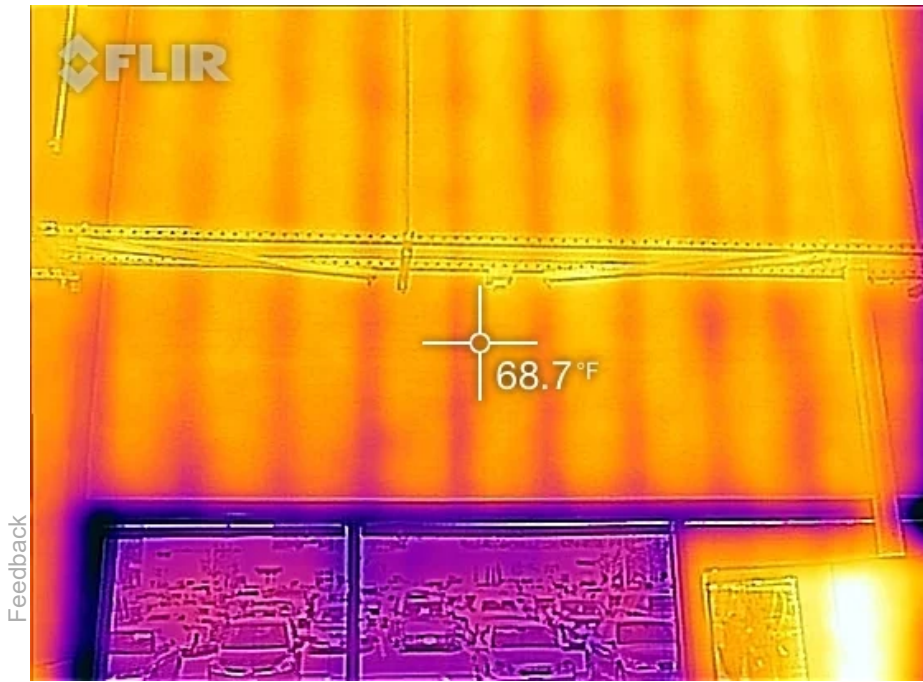
Detecting subtle details, like studs in a wall, requires high thermal sensitivity.
