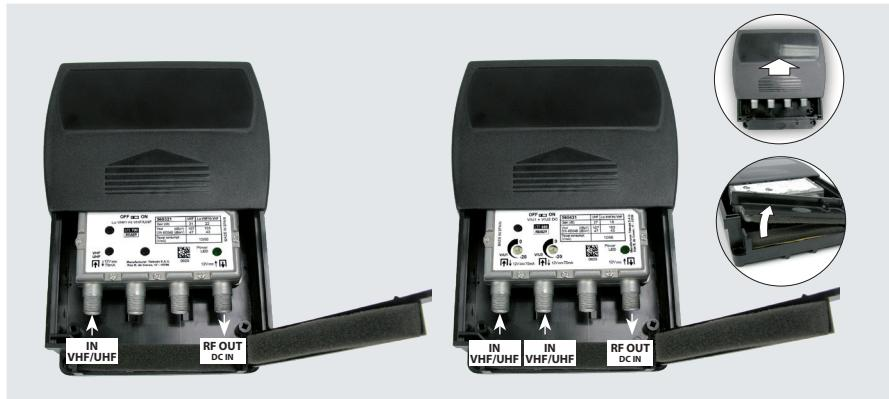
In order to pass 12Vdc power to a pre-amplifier or active antenna ahead of the this pre-amplifier, the switch must be in the ON (right) position. This applies to both the one input and two input model:
