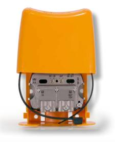
Nanokom masthead amplifier with 1 input (LowVHF/HighVHF/UHF), features a very low noise figure. With the USOS (User Selectable Output Signal) function, the device automatically adjusts its gain to overcome received signal variations based on the user's setting. 12V power supply unit (Ref. 550104) is included.
