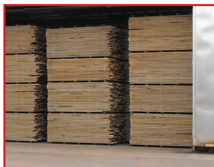
A kiln will dry these hardwood boards to a moisture content of <10%
