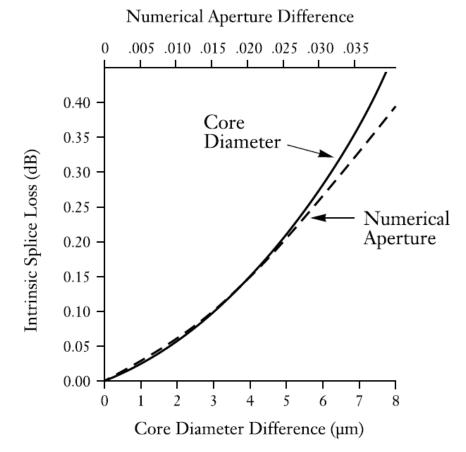
A core diameter mismatch of 5 microns can cause a 0.2dB loss.
