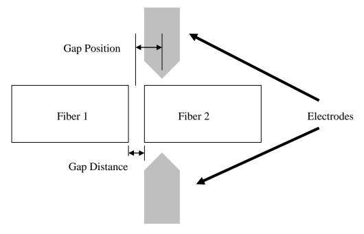
Fiber #1 melts easier so more energy is applied to Fiber #2.
