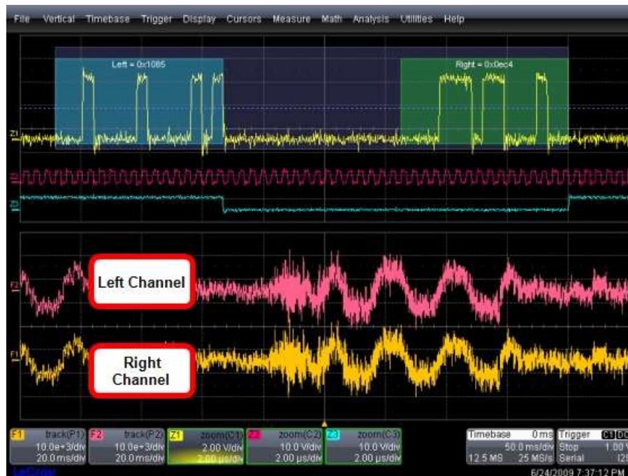
Figure 2: A short zoomed detail of a serial data stream of an audio signal is decoded in the top trace. The two bottom traces are analog waveforms of sound corresponding to the values in the digital waveform
