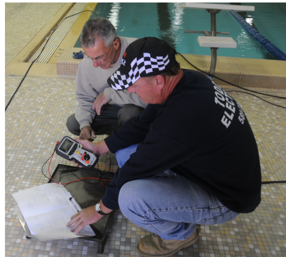
Iaconelli and Art Todd check the reports generated by the Megger MIT420
