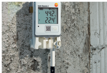
Mould prevention – building humidity (testo Saveris 2-H2 with the digital, external humidity probe 0572 2154)
