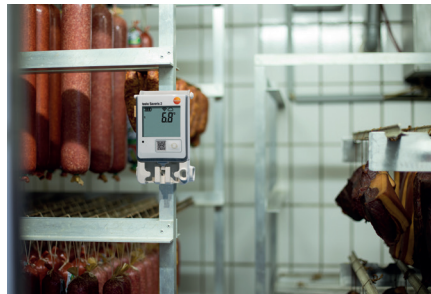
Refrigerated room monitoring at the butcher's (testo Saveris 2-T2 with external NTC probe with door contact)
