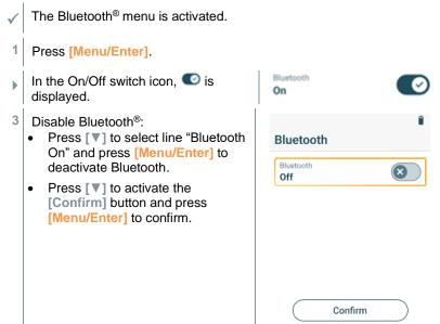
When the Bluetooth<sup>®</sup> icon is not shown on the display, Bluetooth<sup>®</sup> is switched off.
