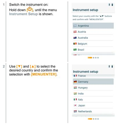
By selecting the country automatically the corresponding area version is activated with different calculation formulas and associated measurement parameters.
