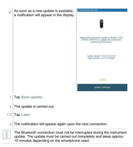
After the update, the measuring instrument will reboot. The firmware can be checked in the instrument menu or via the app. It is recommended to restart the testo Smart App after performing the instrument update.
