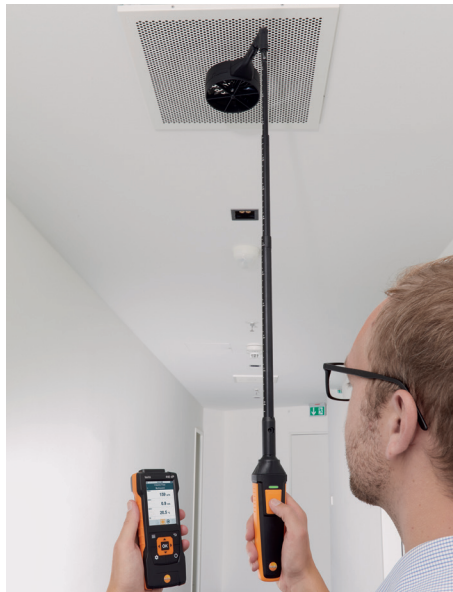
The 4 in. (100 mm) vane probe can be easily combined with the 90° angle and telescopic extension, making measurements at ceiling outlets easier.
