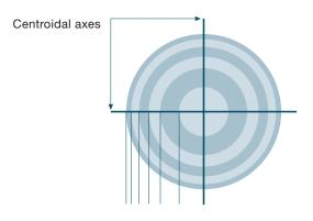
The individual velocity measuring values are used to derive the mean air velocity, from which the volumetric air velocity is then calculated.
