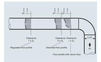
Reduction of irregularity in the flow profile as the clearance from the point of discontinuity increases. Horizontal speed profiles were measured with a Prandtl Pitot tube.
